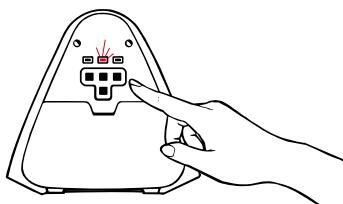
You can program your swing to turn off after a certain period of time. The timer button, located between the two speed buttons, sets the swing time in ten-minute increments up to 40 minutes. Push the button once; the swing will run for ten minutes.
